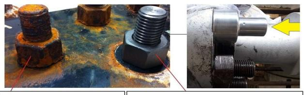
ASTM A193 B7 STUD BOLT + Gr 2H nut EXPOSED TO SALT FOG FOR 600 hours ASTM A193 B7 STUD BOLT + Gr 2H nut EXPOSED TO SALT FOG FOR 600 hours
