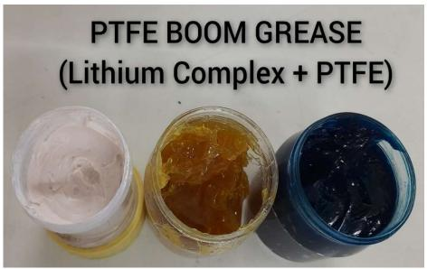
Smooth boom operation on a telescopic crane is a fundamental requirement to all lifting duties. Owing to the construction of modern pinned booms with relatively thin steel sections and large wear pads, this has never been more important. An appropriate lubricant with special properties is required.
